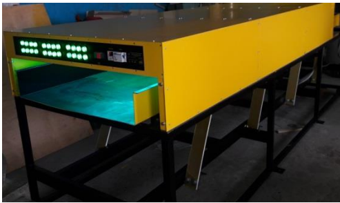
Fig. 2. The OBP10K.2430AS installation conveyor-based with a productivity up to 1000 kg of seeds in an hour.
