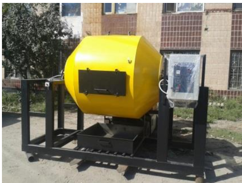
Fig. 1. UV activator of the drum type OBP09.1T10 productivity to 500 kg/h.
